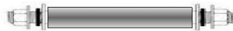
Tie Rod Assembly (Add \frac{1}{2} " Conduit for All Exhaust Duct) And ALL Tie Rods Over 96" in Length
